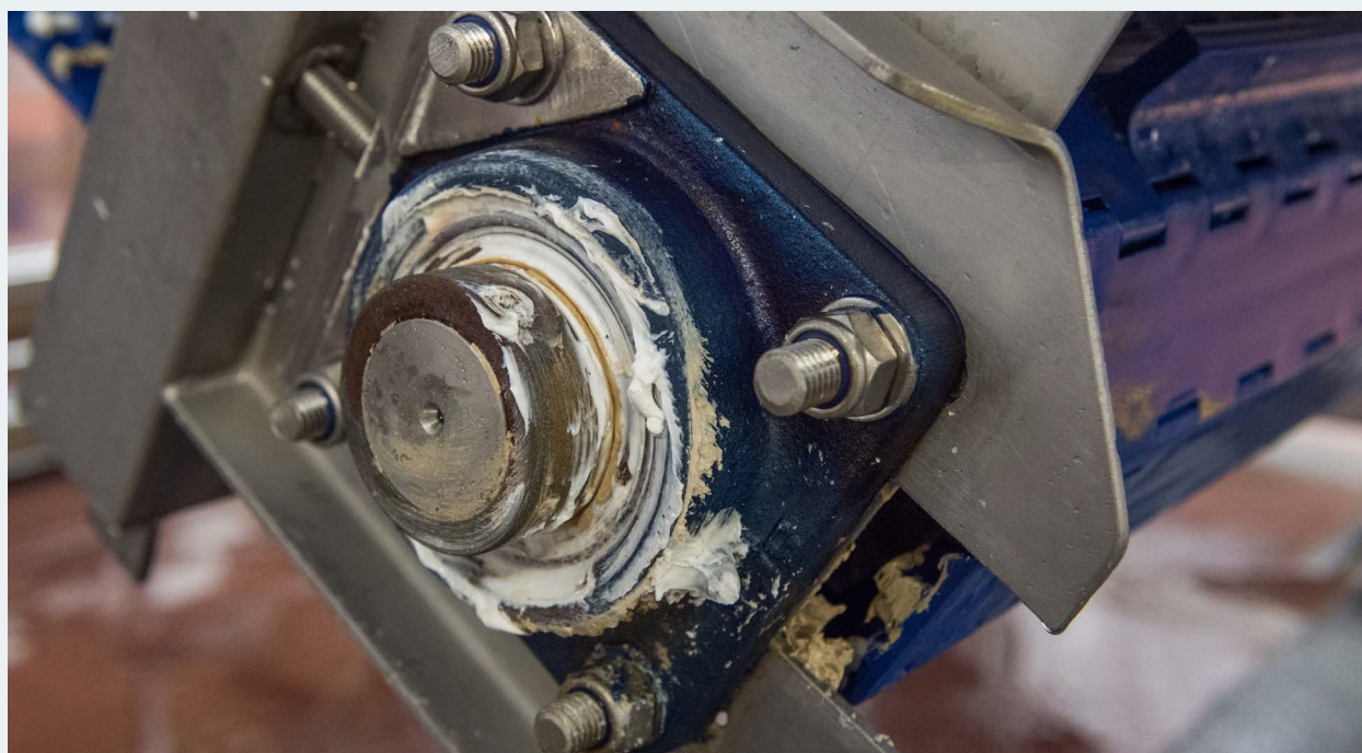
Excess grease from the bearing has collected on the hygienic conveyor belt, increasing the potential for bacteria or allergens to enter the food zone and compromise food safety.
