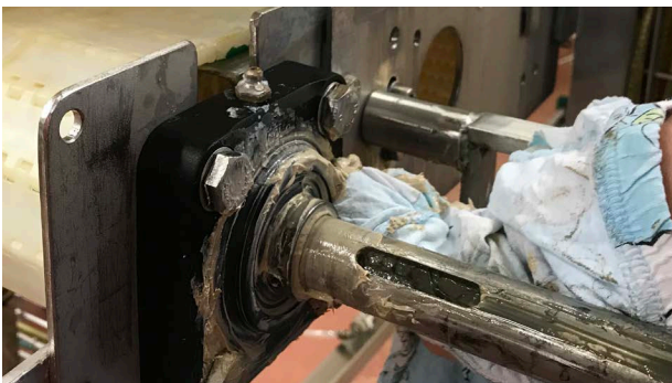
An employee dry cleans grease from a bearing with a cloth that will ultimately be incinerated.
