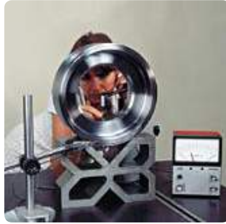
Control and verification instrumentation to measure hardness, dimensions, surface condition, geometrical defects...
