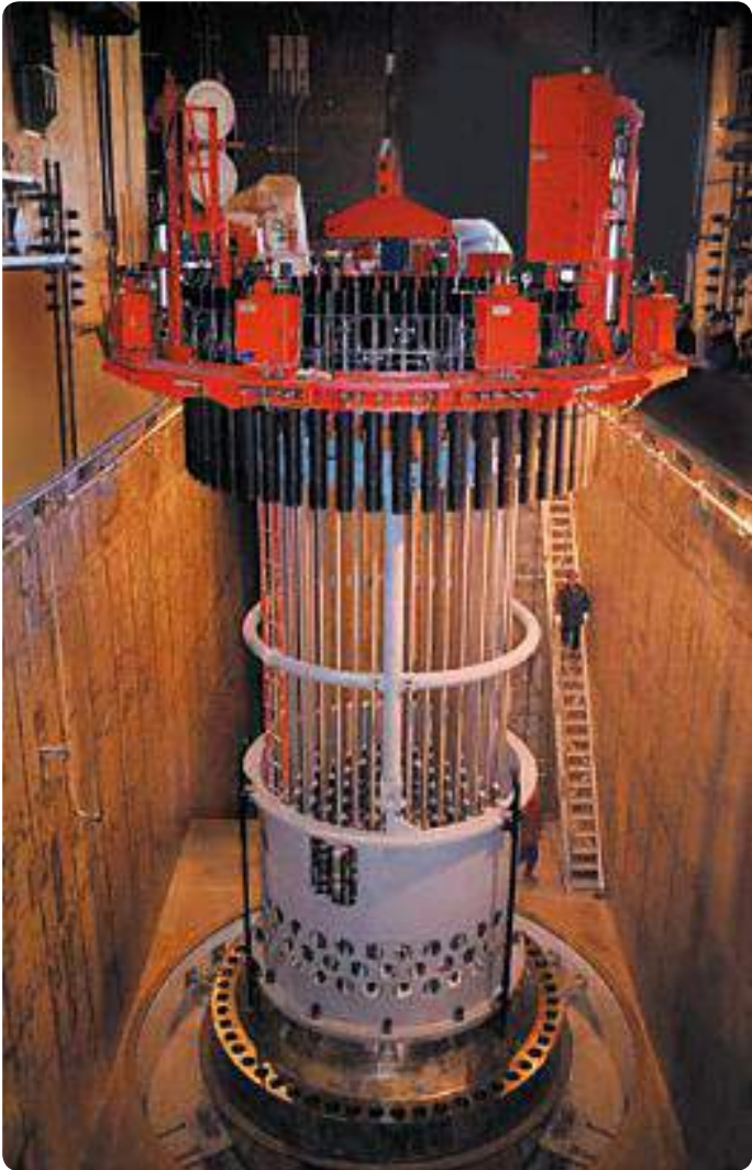
Automatic MST Machine holding 54 vessel studs lowering down to the reactor vessel for closing operation
