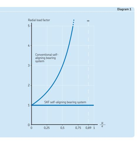
Required radial load for smooth operation of a conventional self-aligning bearing system with two spherical roller bearings, as a function of housing friction
