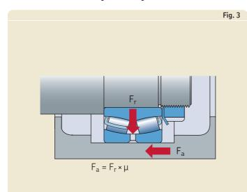
Uneven load distribution is caused by forces emanating from friction in the axial direction
