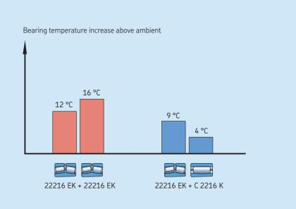
Two other cases of rebuilt industrial fans are shown in **diagrams 4** and **5**. Both examples are conventional centrifugal fans where the spherical roller bearing in the non-locating position was replaced by a CARB toroidal roller bearing of the same size.
