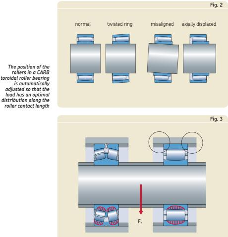
There are no induced axial loads, this ensures even load distribution in both bearings
