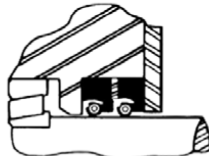
Type HS or HSF seals in tandem arrangement for maximum lubricant retention. Note use of separator between seal elements.
