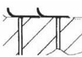
Two sleeves for double seal installation.
