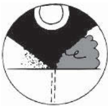
Conventional trimmed lip has sharp edge & rough surface on lube side.
