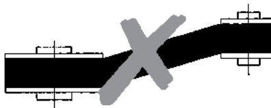
Axial misalignment of sheaves
