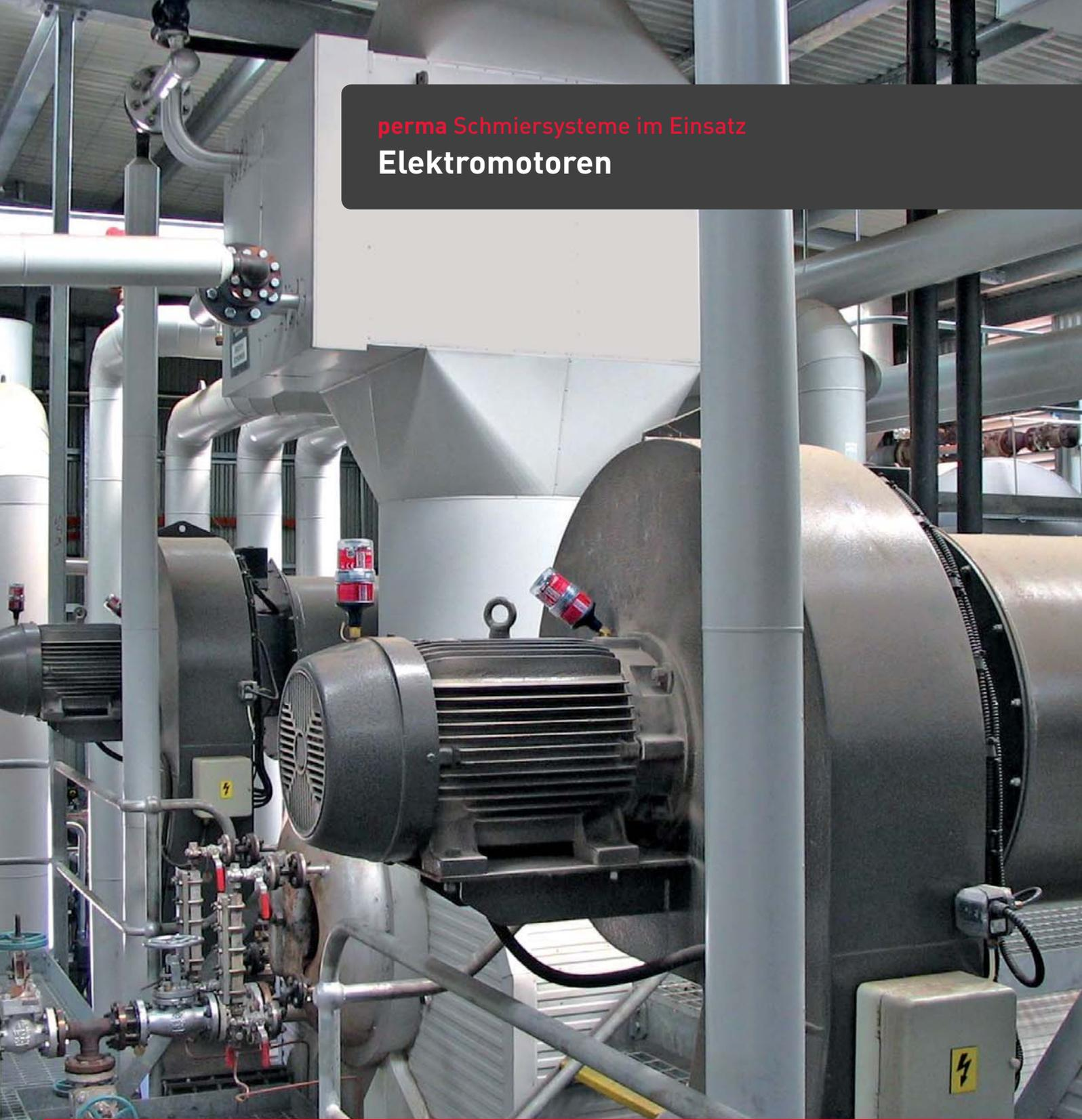
A photograph of an industrial facility, likely a power plant or refinery, featuring several large electric motors and complex piping systems. The scene is brightly lit, showing metallic surfaces and various pipes. Two red Perma automatic lubrication systems are visible, one mounted on a motor and another on a large cylindrical component. Electrical control boxes with warning symbols are also present.
