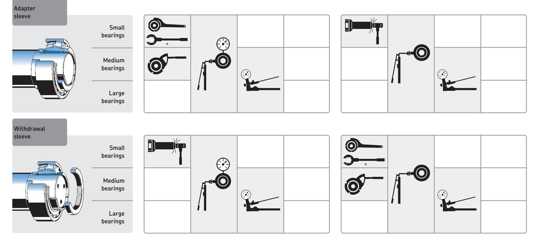
Small bearings: Bore diameter < 80 mm / Medium bearings: Bore diameter 80 – 200 mm / Large bearings: Bore diameter > 200 mm / \* Only for self-aligning ball bearings.
