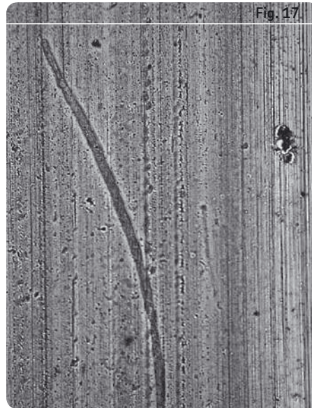
Indentations in the raceway caused by over-rolled contaminants
