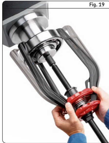
Mechanical jaw puller with spring operated arms
