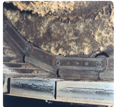
Chain grate furnace
